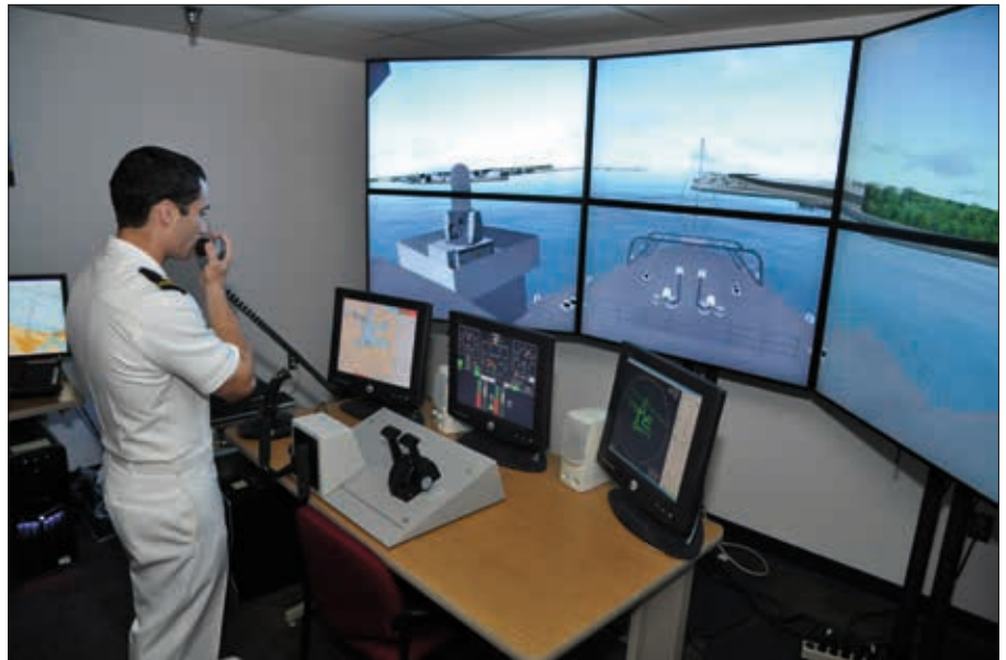
Sailor assigned to amphibious transport dock ship USS Ponce uses voice-recognition system to command virtual simulation of Ponce in Conning Officer Virtual Environment (U.S. Navy/Nathanael Miller)
