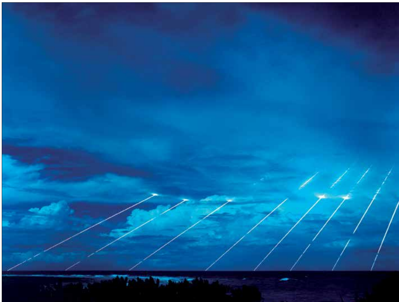
LGM-118A Peacekeeper missile system tested at Kwajalein Atoll in Marshall Islands shows paths of multiple re-entry vehicles deployed by missile (U.S. Army/David James Paquin)
