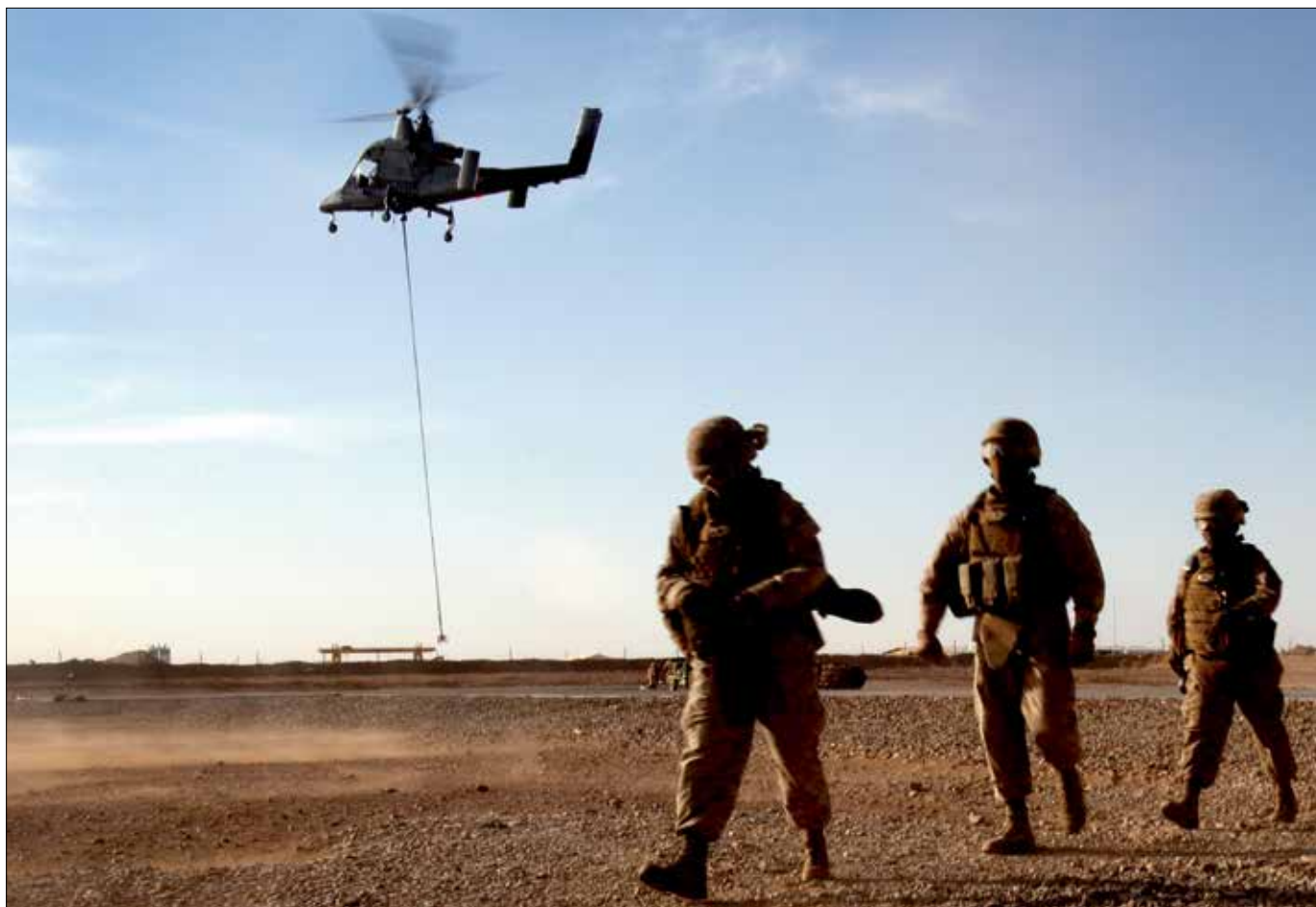
Marines with Combat Logistics Battalion 5 return after learning about downward thrust of Kaman K1200 ("K-MAX") unmanned helicopter during initial testing in Helmand Province, Afghanistan (U.S. Marine Corps/Lisa Tourtelot)
