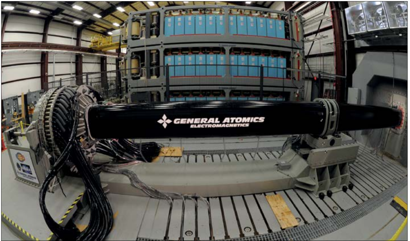
Electromagnetic Railgun launches projectiles using electricity instead of chemical propellants for use aboard ships, June 21, 2012 (U.S. Navy/John F. Williams)
