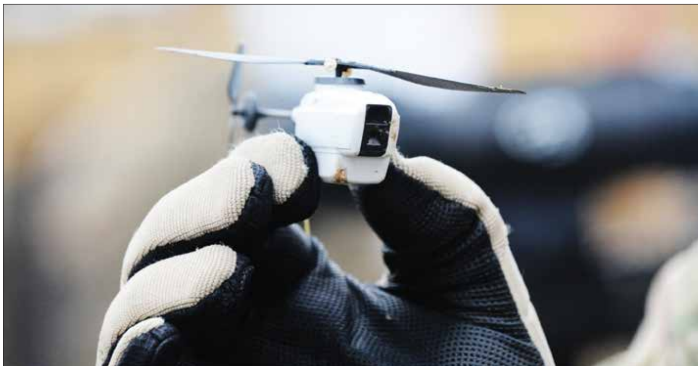
Researchers with U.S. Army Natick Soldier Research, Development, and Engineering Center are testing Prox Dynamics PD-100 Black Hornet Personal Reconnaissance System to provide squad-size units with organic aerial ISR capability in challenging ground environments (Courtesy UK Ministry of Defence)
