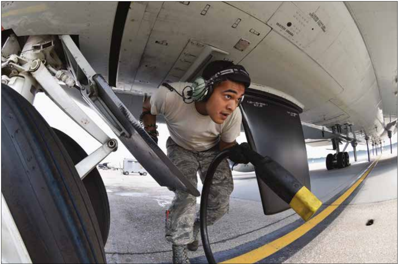
Senior Airman with 55 th Aircraft Maintenance Squadron disconnects external power cord from extensively modified RC-135V/W Rivet Joint, with onboard sensor suite allowing mission crew to detect, identify, and geolocate signals throughout electromagnetic spectrum, August 5, 2018, at Offutt Air Force Base, Nebraska (U.S. Air Force/Drew Nystrom)
