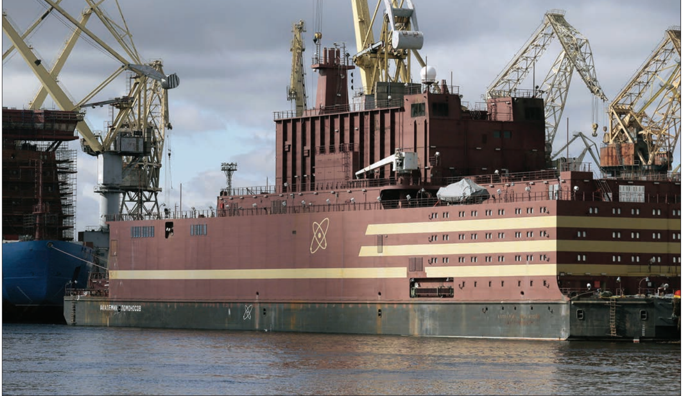
Russia's floating nuclear power barge Akademik Lomonosov , with two nuclear reactors with capacity of 35 megawatts each, leaves Saint Petersburg under tow for Murmansk, April 28, 2018 (NurPhoto/Valya Egorshin)
